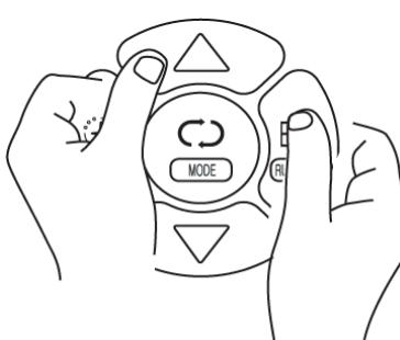
Set the required temperature and switch on the heating. Switch on the automatic tuning while holding down the  $\Delta$  and ENT buttons for 3 seconds. The operation can be interrupted by pressing this button combination once again.
