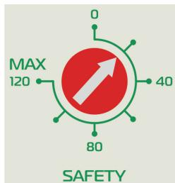
User must set the over temperature protection before operation.
